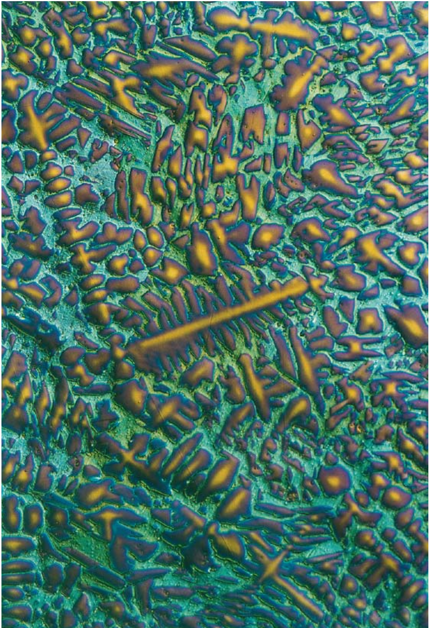
AS CAST TIN BRONZE, MAGNIFICATION 300x
