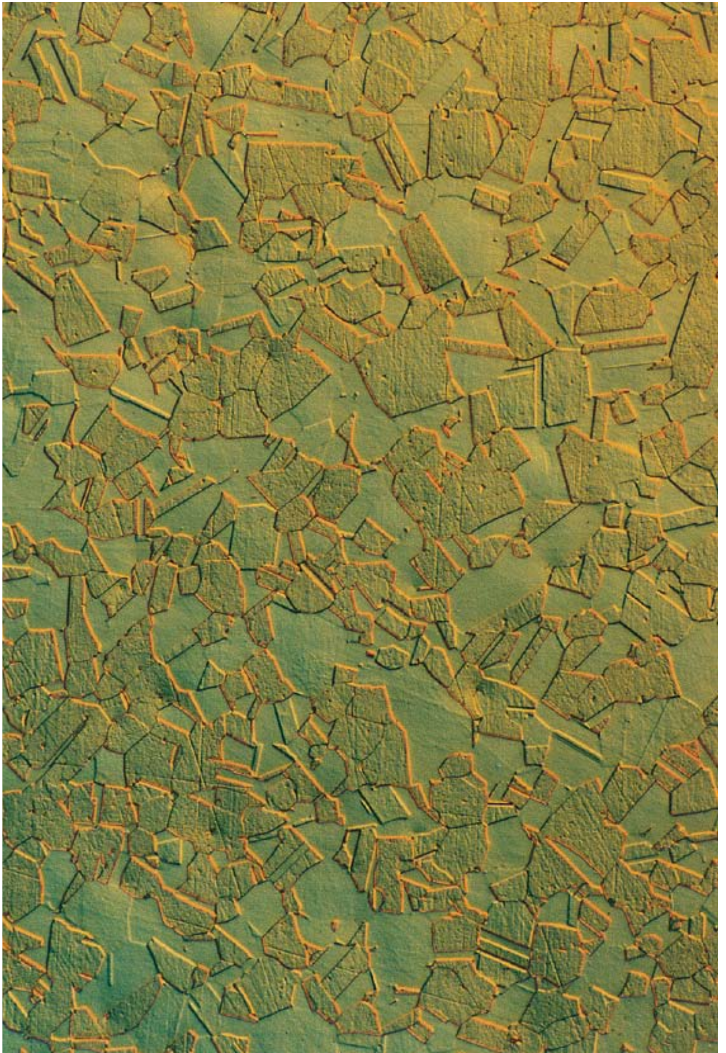
UNLEADED BRASS, MAGNIFICATION 200x
