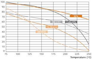
This new material is a copper matrix alloy containing nickel and tin. A small amount of lead is added to improve the machinability. This alloy is absolutely free of beryllium which minimizes any ecological impact and allows the easy recycling of chips resulting of free machining operations.
